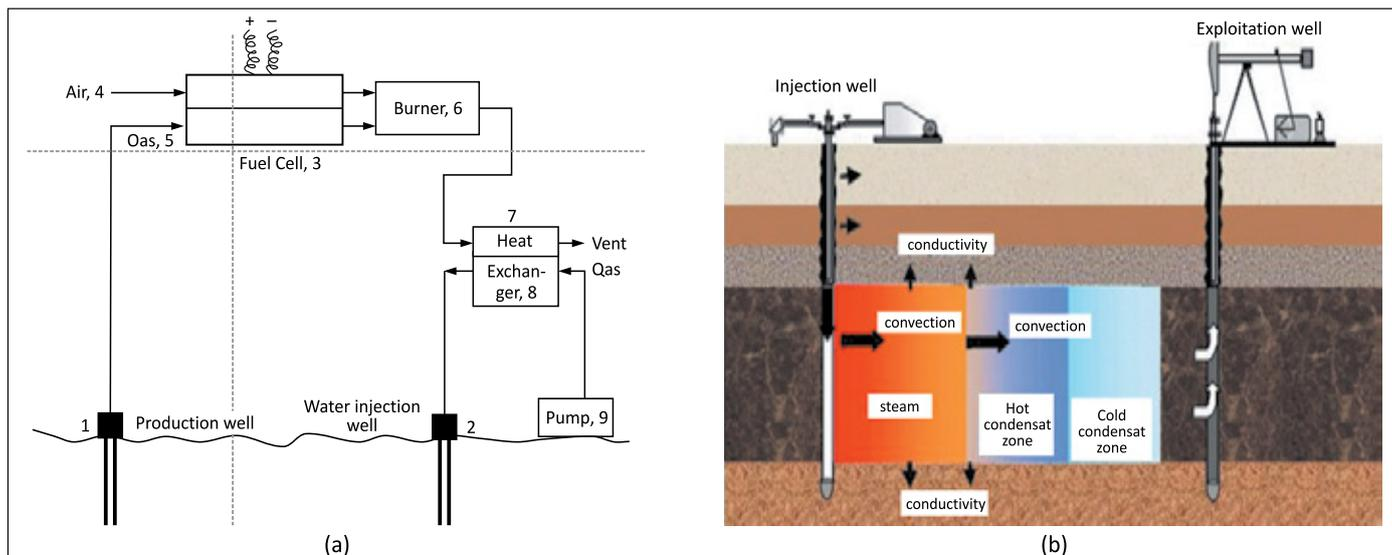
**Figure 4.** Scheme of fuel and energy production device using a fuel cell surface installation (a) and implementation of the Thermolift technology in the well (b)
